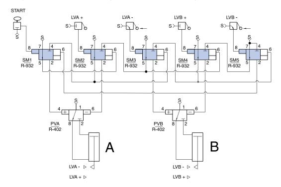
NOTE: The SEQUENCE IS FOLLOWED by the indicator in the valve. The last indicator down is the last step actuated. This is helpful when trouble shooting a circuit.
